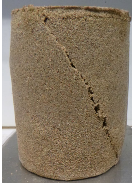
Figure 10. Sand specimen at the end of the triaxial test T1 at \sigma_3 = 0.3 MPa; \dot{\epsilon} = 0.1 %/min.
