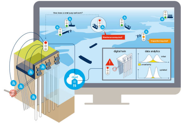
Figure 2. Concept of a smart quay wall (Roubos, 2019).
