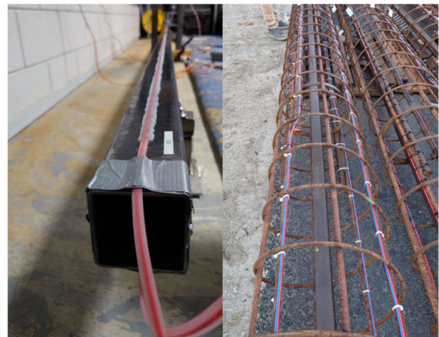
Figure 4. Impression fibre optic strain sensors.
