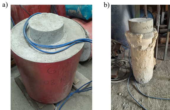
Figure 5. The pile shaft model before (a) and after (b) testing.
