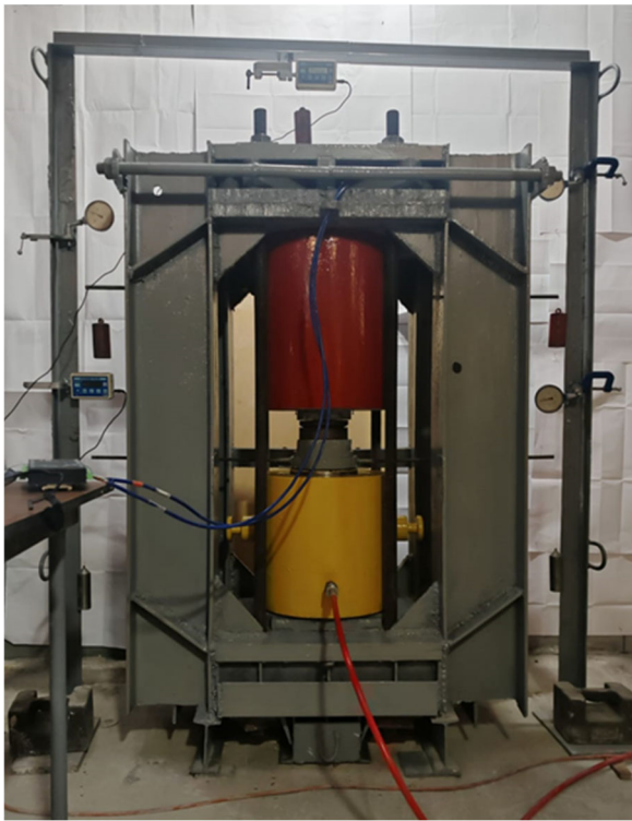
Figure 4. Pile shaft model installed in a special load frame.
