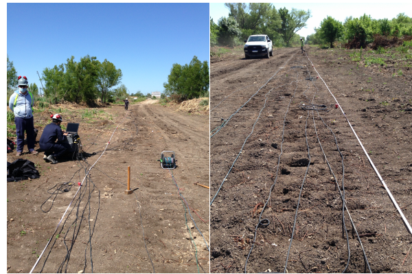
Figure 5. Typical layout for geophysical test (tape 100 m, cables, geophones 4.5 Hz, hard-soft unit and 6 kg sledgehammer).
