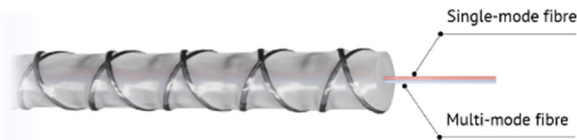
Figure 10. Distributed strain sensor (EpsilonSensor) with two fibres for simultaneous strain and temperature measurements.
