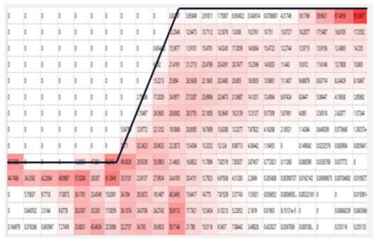
Figure 10. Example plot of multi-zone optimization Areas of darker red indicate areas where higher levels of additional strength are needed.
