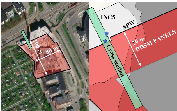
Figure 1. Overview of the Campus Ullevål excavation pit, showing the location of inclinometer INC 5 and the cross-section selected for numerical analysis.
