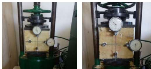
Figure 7. Uniaxial compression test of limestone specimens
