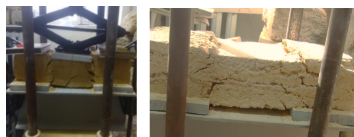
Figure 6. Punching test of limestone samples
