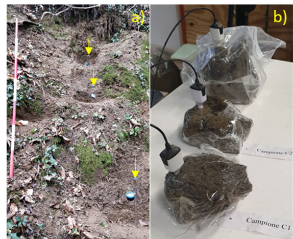
Figure 5. Suction measurements that were carried out: a) in-situ with jet-fill tensiometers; and b) in the laboratory with digital mini-tensiometers.
