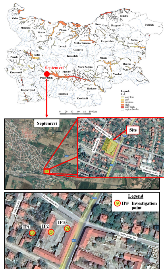
Figure 1. Regional and site location: (top) liquefaction hazard zones in Bulgaria with project site – (Nakov & Dobrev, 2014); (middle) satellite view; (bottom) site plan with investigation points.
