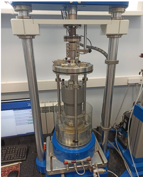
Figure 7. The torsional ring shear apparatus during testing.
