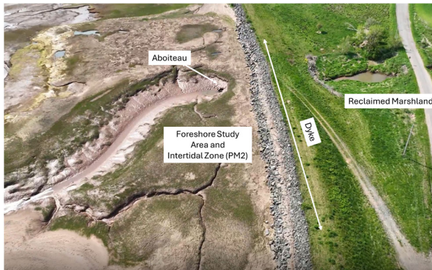
Figure 1. Drone photo of study site. Dyke crest is approximately 3 to 4 m wide for scale.
