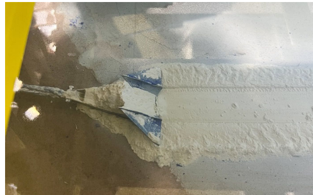
Figure 11: Failed Test 4a in which the anchor rotated onto its back.
