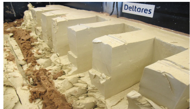
Figure 8: Clay sample after exhumation without anchors (side view).
