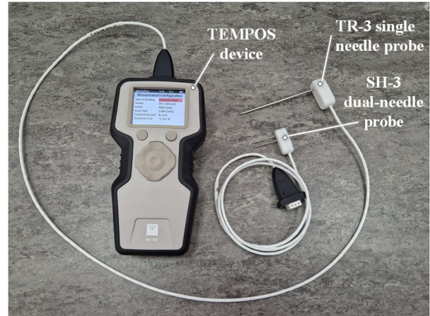
Figure 1. TEMPOS Thermal Properties device along with the two needle probes.
