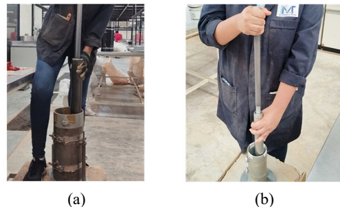
Figure 5. Compaction of specimens. (a) Samples of 15 cm in diameter and (b) Samples of 7.1 cm in diameter.
