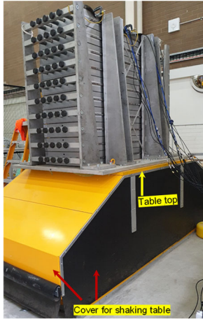
Figure 1. Laminated shear stack placed on the biaxial shaking table at UNSW.
