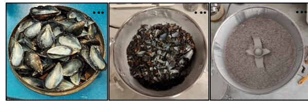
Figure 1. a) the mussel shell; b) mussel shell granule; c) mussel shell powder.
