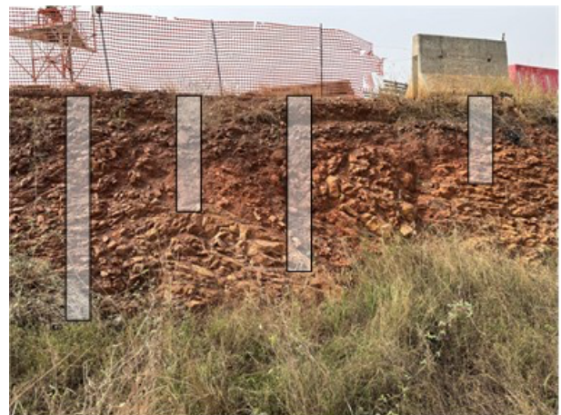
Figure 2. Phyllite bedrock variability exposed in a cutting close to the ATC tower site.
