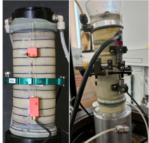
Figure 3. (Left) Hall-effect sensors (Antea group laboratory) and (Right) LVDT (EDF laboratory) sensors after testing.
