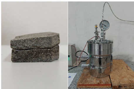
Figure 2. a. Discontinuity specimen. b. Carbonation cell.
