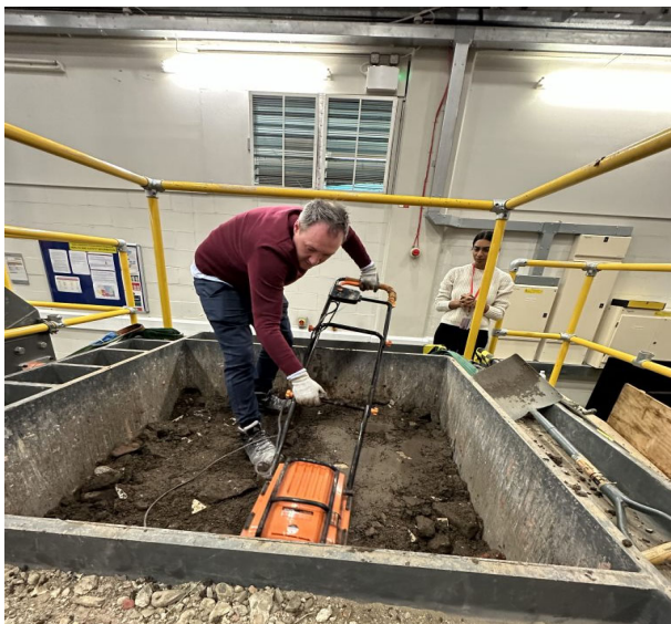
Figure 3. Compaction of a layer using a small wacker plate.
