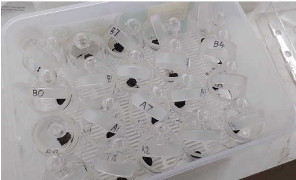
Figure 5. Small soil fragments in glass weighing bottles.
