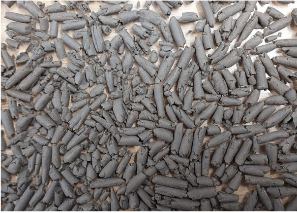
Figure 4. Soil thread after rolled to crumbling state.
