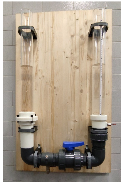
Figure 1. Test apparatus designed for the determination of water permeability normal to the plane of geotextiles GTX and drainage geocomposites GCD.
