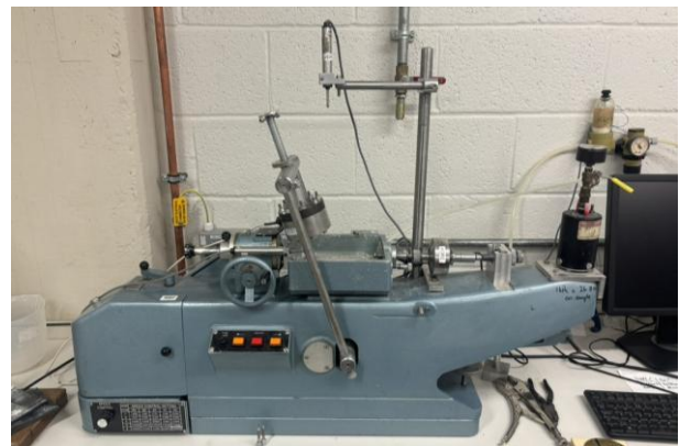
Figure 1. Standard direct shear box test apparatus at City St George's, University of London.
