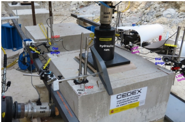
Figure 11. Arrangement of the monitoring system
