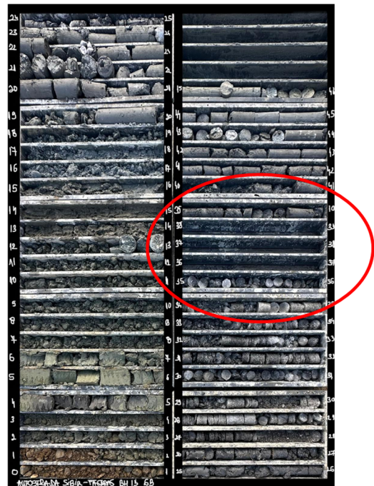
Figure 3: Interlayered salt and gap in the layers, borehole 45m depth (Milutinovici, et al., 2024)
