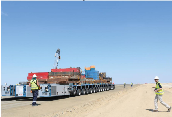
Figure 4. Test trailer for the dynamic embankment trial
