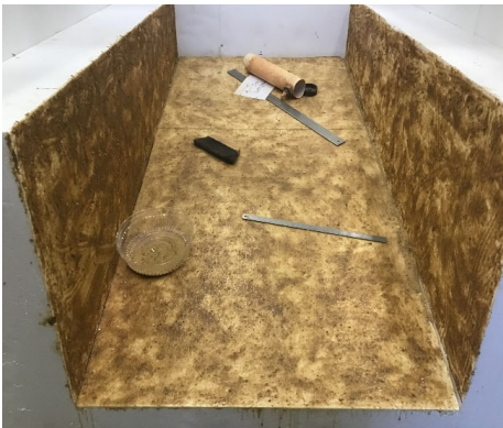
Figure 3. The container for the experiments was created using EPS foam blocks coated with sanded epoxy. A rigid wooden frame was used to hold the EPS in place (not shown in the photo).
