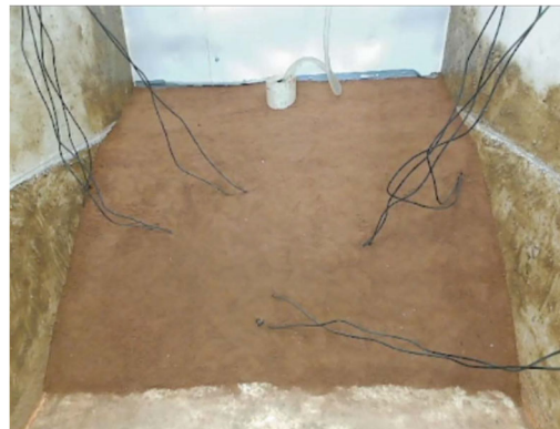
Figure 4. Completed slope after pipe removal, but before testing. The standpipe is shown at the top of the slope along with the tube used to introduce flow into the pipe.
