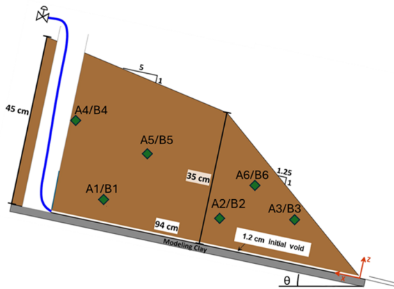
Figure 2. Cross-section of the model showing the sensors' location. The locations of the sensors (A1/B1 – A6/B6) are indicated by green diamonds. The width of the model (y-direction) is 120 cm.
