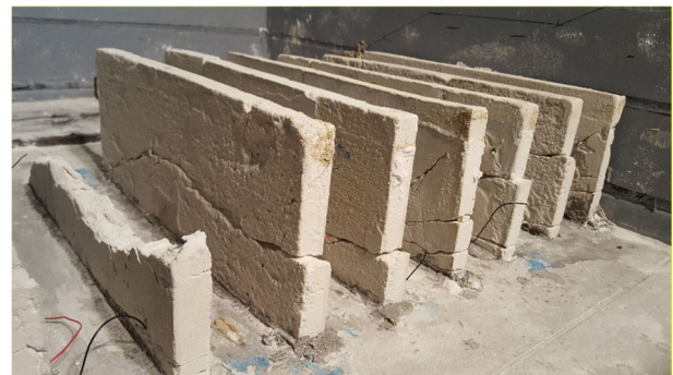
Figure 8. Post-test excavation photo of soil-cement walls from the embankment side looking toward the toe (Boulangier et al. 2018)
