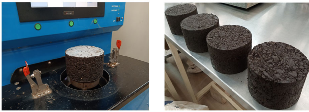
Figure 9. Compaction of specimens in gyratory compactor.
