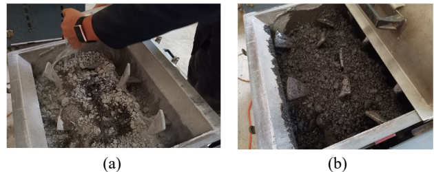
Figure 7. (a) Adding 75% of water, (b) Mixing aggregate-lime-water.
