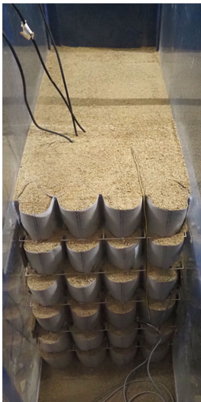
Figure 2. Photograph of the geocell-GAC retaining wall model
