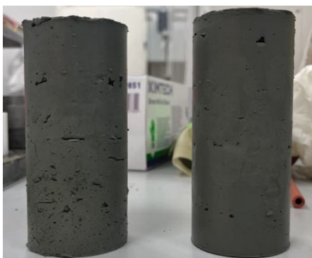
Figure 4. Observation of more air pockets and less compaction in the top half of sample tube (left) in comparison to the bottom half of sample tube (right).
