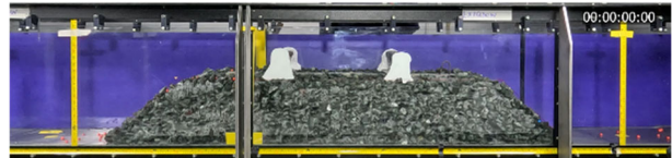
Figure 5 Installed ballast specimen in the open-channel flume before testing
