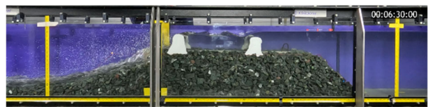
Figure 6 Ballast specimen in the open-channel flume after testing (30 m 3 /h)
