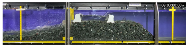
Figure 7 Ballast specimen in the open-channel flume after testing (40 m 3 /h)
