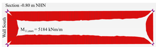
Figure 13. Horizontal section through the D-walls at z = -0.80 m for the maximum bending moments.
