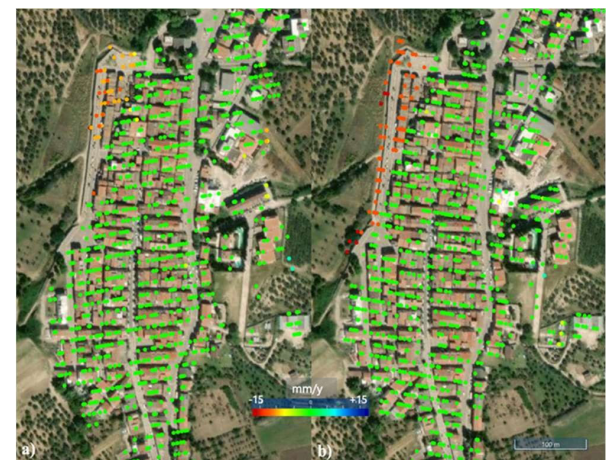
Figure 3. a) Ascending and b) descending mean velocity maps resulting from the processing of the CSK datasets between January 2015 and December 2020 (Sonnessa et al., 2023).
