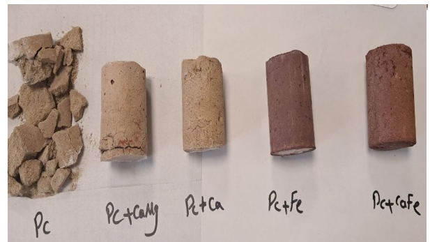
Figure 3. PC and PC-carbonate-treated samples in the sulfate attack test.
