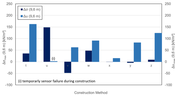
Figure 6. Permanent change of total horizontal earth pressure and temporary excess pore water pressure at 9.6. m bgl. due to construction.
