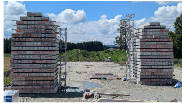
Figure 4. Group zone load tests including shallow foundation are shown in loading step 3.
