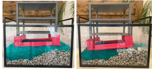
Figure 10. Scale model, differential settlement caused by regional subsidence and irregular basement, before and after leveling
