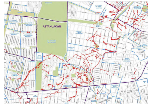
Figure 3. Map of cracks in “Santa Cruz Meyehualco” and “Santa María Aztahuacán”. (Auvinet, et al., 2020)
