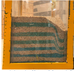
Figure 8. Physical model and effect of funnel flow in the sand
