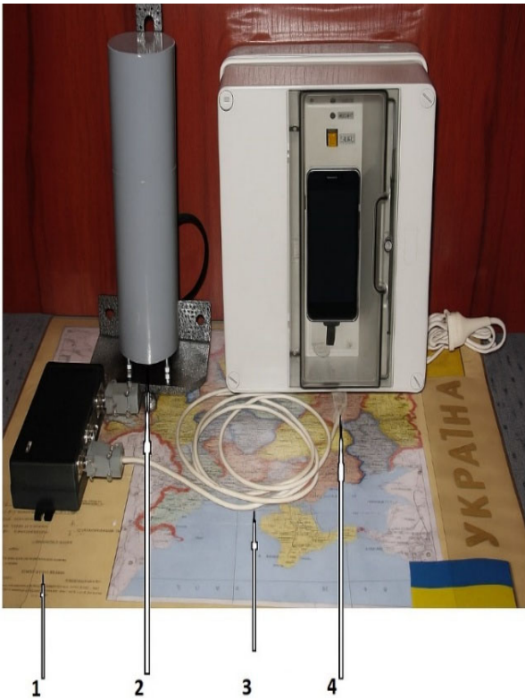
Figure 1. Technical means of the automated measuring and information system: 1 – inductance meter; 2 – sensor for measuring angular deformations; 3 – communication lines; 4 – unit for collecting and transmitting information to the cloud.
