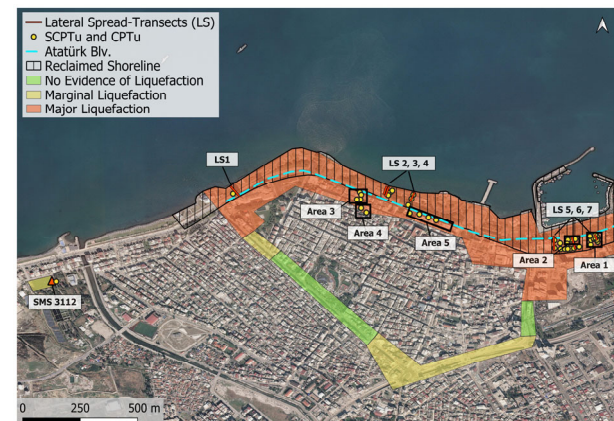
Figure 2. Overview of İskenderun study areas with demarcation of reclaimed and historic shoreline boundaries from Arnold et al. (2025).
