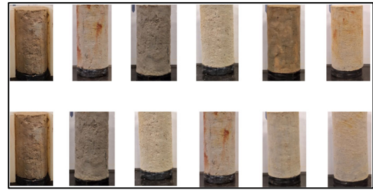
Figure 3. Trimmed soil samples.
