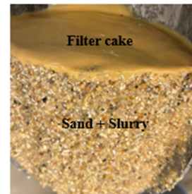
Figure 5. Photo of the surface cake and the internal deposition of the bentonite fluid particles
