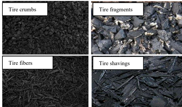
Figure 7. Products from the Processing of End-of-Life Tyres (Edinçliler, Baykal e Saygili, 2010; Araújo, 2023).
