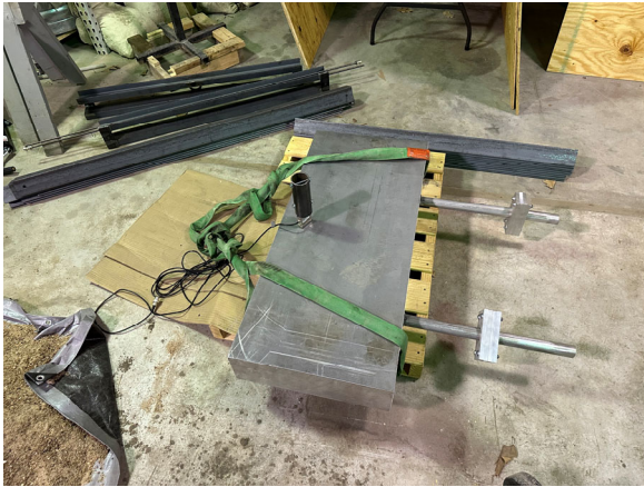
Figure 2. Abutment, piles, and load cell
