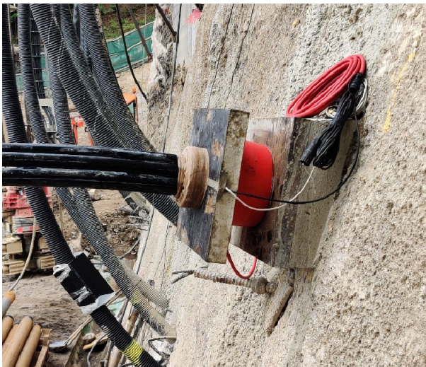
Figure 7. Test anchor using conventional electronic load cell
