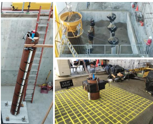
Figure 2. Construction photos (left: test pile secured in the Soil Pit; top right: sand pluviation; bottom right: during testing).
