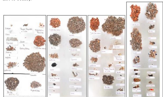
Figure 3. Separation of materials from samples RCC1, RCC2, RCC3, and RCC4 (from left to right) (representation not to scale).
