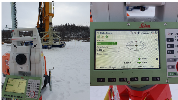
Figure 5: Leica Total Station TS16 (left) and Stake Points Screen TS16 (right)
