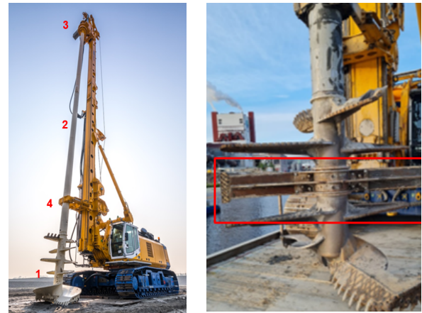
Figure 4: Main equipment BG45 (left), optimized mixing tool with static bar (right)
