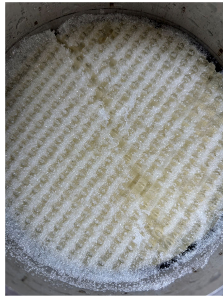
Figure 13. Image for upper part of the 3D filter with 4.8mm wire diameter for GB-I.
