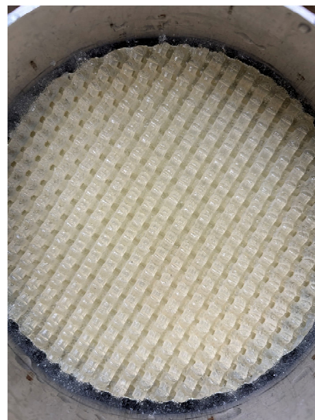
Figure 14. Image for upper part of the 3D filter with 4.8mm wire diameter for GB-II.
