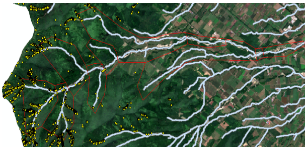
Figure 6. Source of driftwood from slope failures in the Memuro river basin (yellow points).
